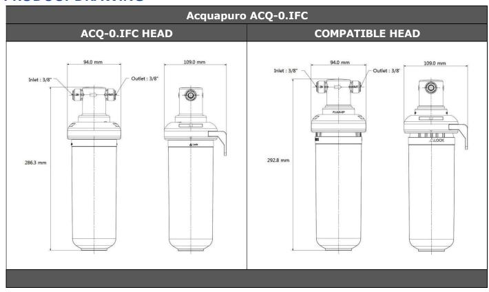
The left product is the ACQ-0.IFC filter and head, the right product is a compatible head with the Acquapuro ACQ-0.IFC filter.
