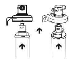
4. Hold head firmly. Insert new cartridge into the filter head.
