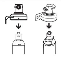
3. Pull cartridge down and out of head.
