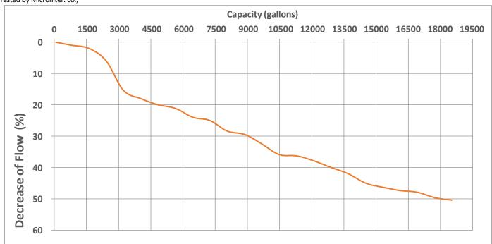
This is a test for the Acquapuro ACQ-0.IFC filter, results may vary according to flow rate influent line pressure and local water conditions. For detailed filter performance, please refer to the page.6 data sheet.
